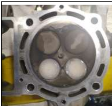
Check the flatness of cylinder head with a stopper
