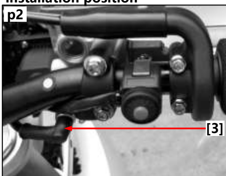
p2: factory edition Brake switch installation position
